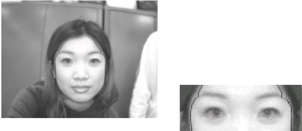
Figure 9.5: Demonstration of step 5 - second edge detection. Notice that the second time the edges are found accurately.
