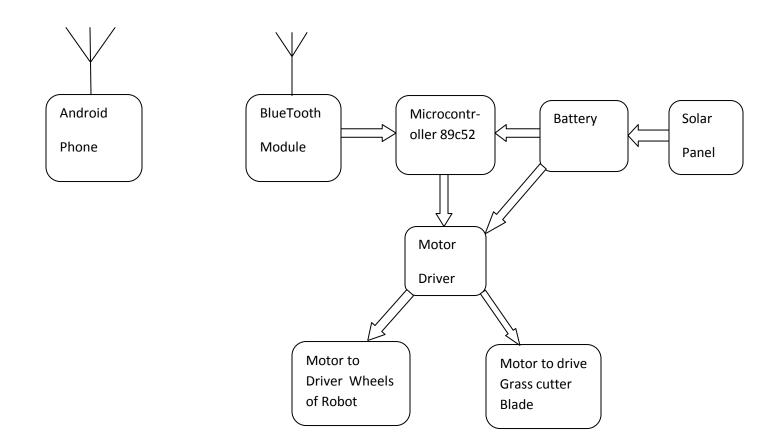
Figure shows block diagram of solar based grass cutter robot. The robot is getting control by android phone. By using android phone we can transfer data to Bluetooth module. The data from Bluetooth module is received by controller and take action according to data. Controller controls the motor revolution as per data. The robot will get the power from solar panel. When ample sun energy is available it is stored in battery. When sun energy is not available, stored energy in the battery is used.
