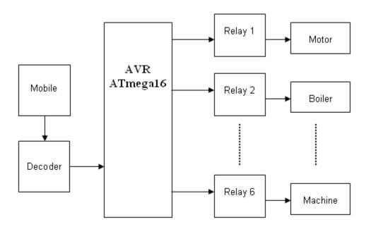
**Description:** For giving command, you have to just call on the mobile on set which you have set on field. This mobile is on auto answering mode. This will receive your call. Then particular key is assigned to every controlling action. E.g. - key 1- turn on motor, key 2- turn off motor. Key 3- turn on machine etc. Such that by giving commands from mobile you can control industrial work. It is advantages for all type of industrial work.
