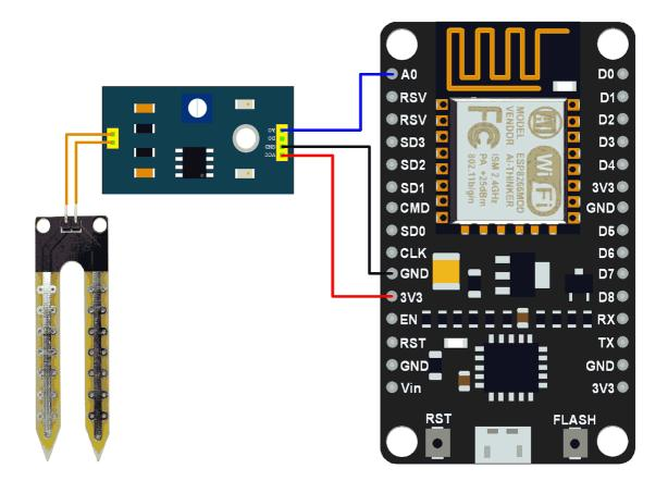
Most soil moisture sensors are designed to estimate soil volumetric water content based on the dielectric constant (soil bulk permittivity) of the soil. The dielectric constant can be thought of as the soil's ability to transmit electricity. The dielectric constant of soil increases as the water content of the soil increases..
