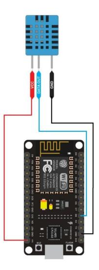
DHT11 is a Humidity and Temperature Sensor, which generates calibrated digital output. DHT11 can be interface with any microcontroller like Arduino, Raspberry Pi, etc. and get instantaneous results. DHT11 is a low cost humidity and temperature sensor which provides high reliability and long term stability
